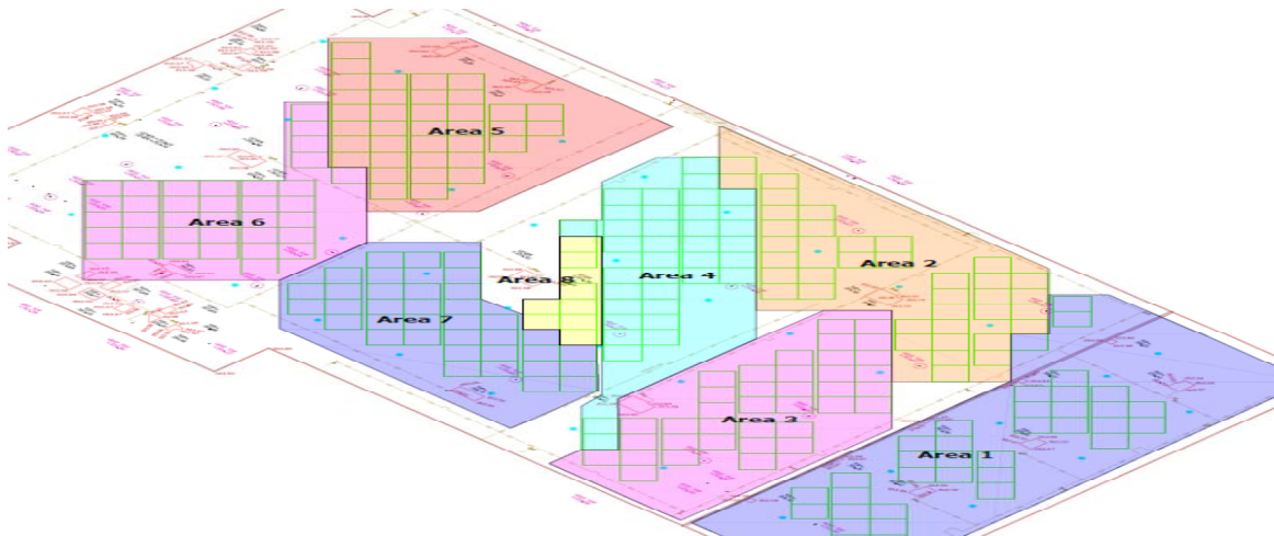
Figure 22: Sample PowerTilt Installation Sequencing Plan
