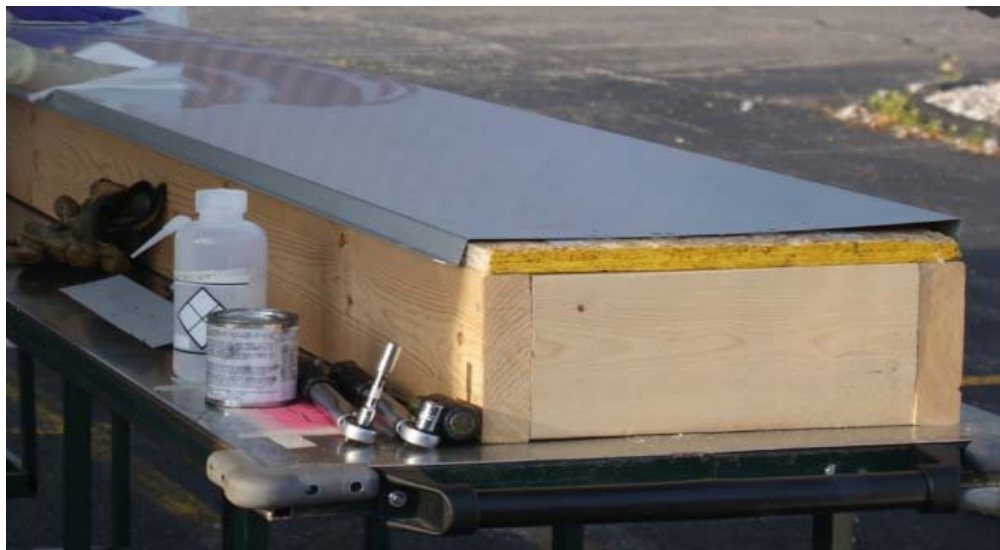
Figure 4 Lamination Work Station and Metal Pan Wooden Template
